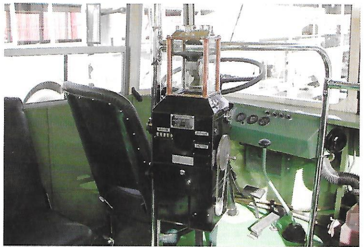
The restored driver's area of bus 8 retains an authentic dash and controls. The fare box is typical of those used in small buses on rural routes.
